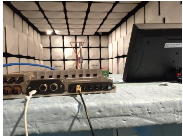
Radiated measurements with antenna type Interior WLAN
