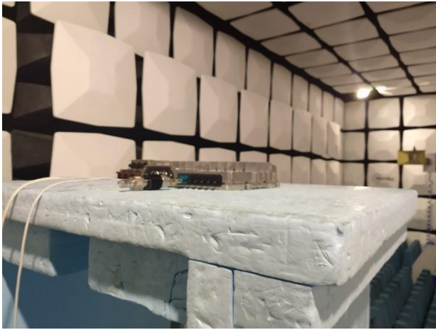
Radiated measurements with 50ohm termination
