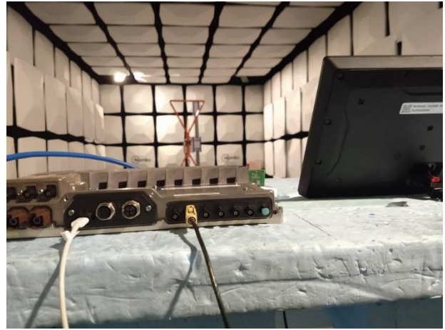
Radiated measurements with antenna type Interior WLAN
