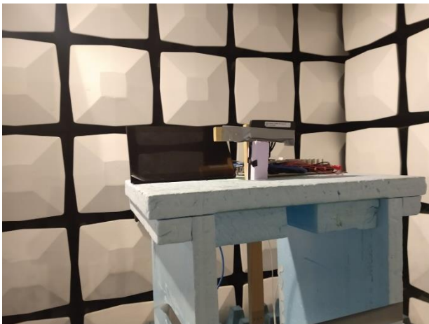
Radiated measurements with antenna type 2J
