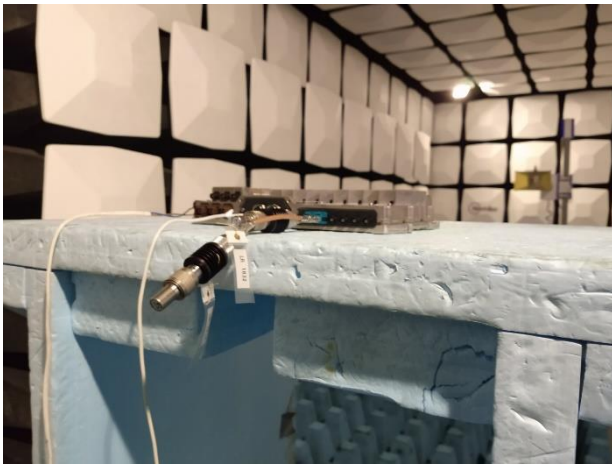
Radiated measurements with 50ohm termination
