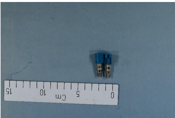
FAKRA to SMA RF connector for conducted test
