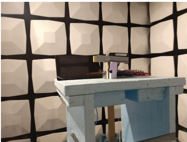
Radiated measurements with antenna type 2J
