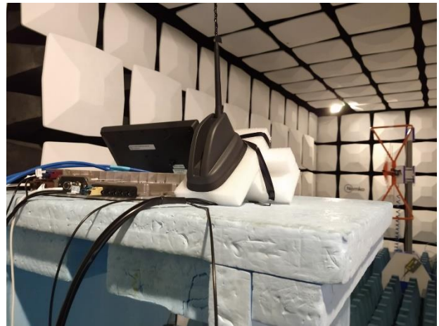
Radiated measurements with antenna type Base
