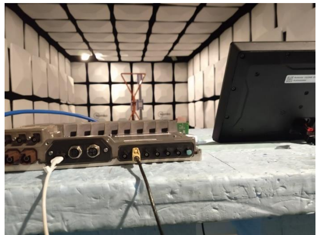
Radiated measurements with antenna type Interior WLAN
